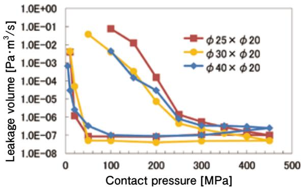
(b) Relationship between leak rate and contact gasket stress for copper flat gaskets
