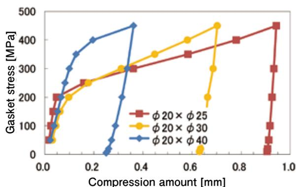
(b) Compression properties of copper flat gaskets
