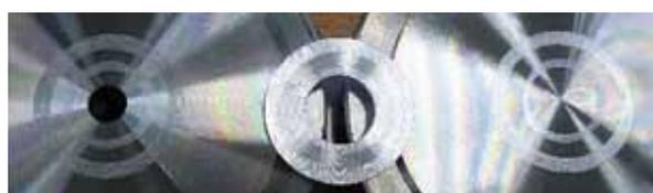
Figure5 Surfaces of gasket and flanges after compression test
