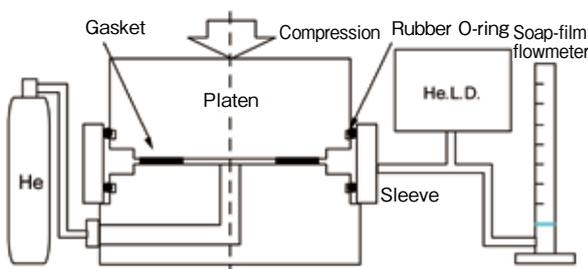
Figure2 Illustration of platen test equipment
