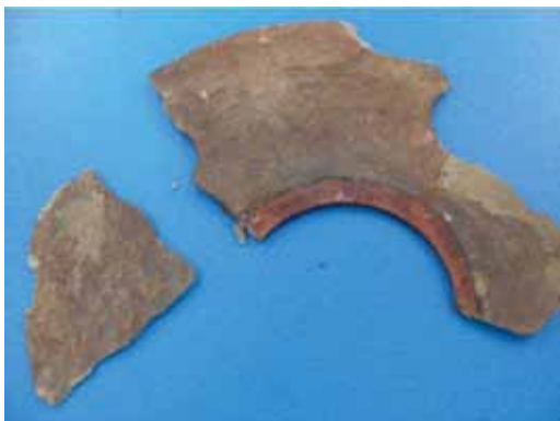
Figure5 压缩板的硬化开裂
