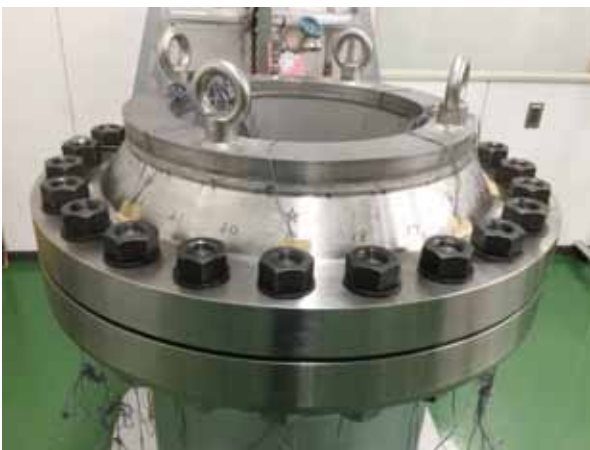
Figure3 24-inch flange connection
