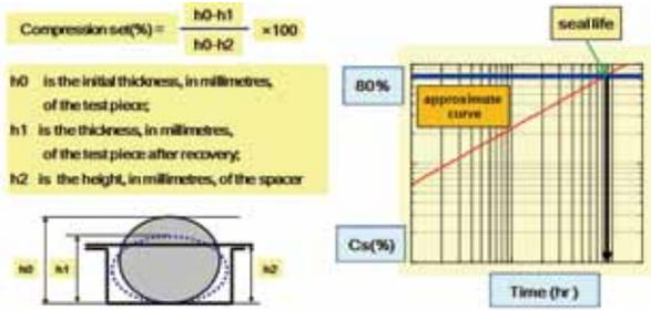
Figure3 Compression-set test and expected lifespan
