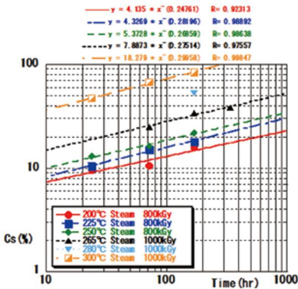
Figure7 A plot of the results of compression-set tests
