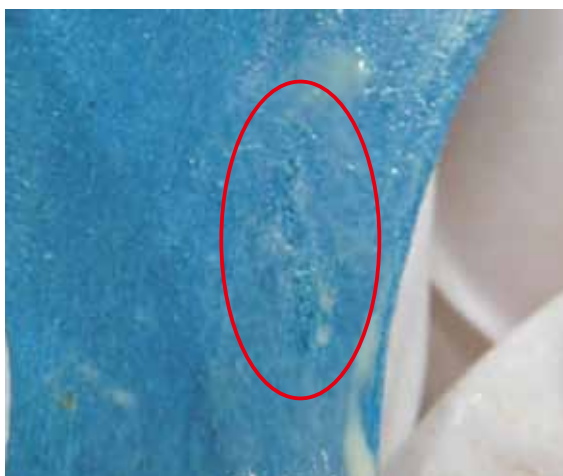
Figure 4 Compression-fracture test of improved seal paste Compression fracture was confirmed at 100 MPa.
