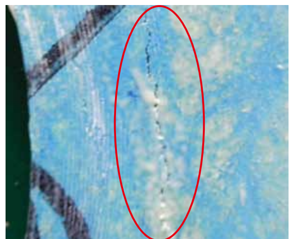
Figure 3 Compression-fracture test of conventional seal paste Compression fracture was confirmed at 100 MPa.
