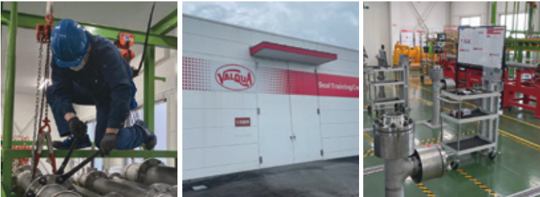
Exterior of, and impression of practical training at, the experience-based training facility Seal Training Center (STC) (Left: Impression of on-site simulated tightening training, Center: STC exterior, Right: Example of training device)
