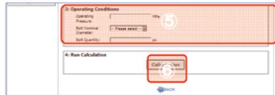
⑤ Input the operating pressure, bolt nominal diameter, and bolt quantity, which are to be calculated.
