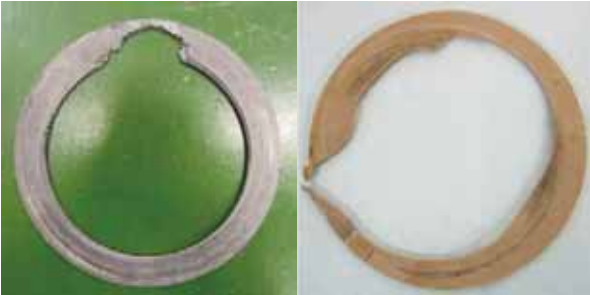
Figure3 Erosion of a soft gasket
