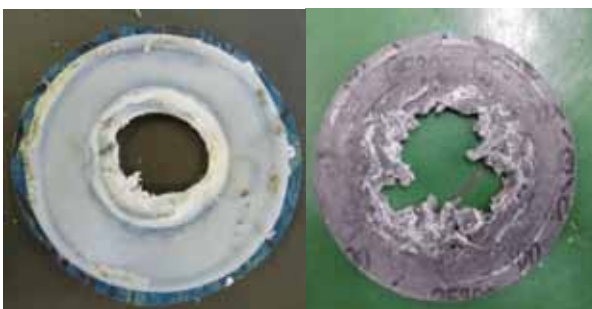
Figure1 Blooming phenomena of a resin-type gasket
