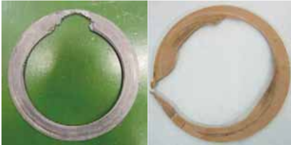
Figure3 Erosion of a soft gasket
