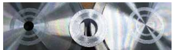
Figure 5 Surfaces of gasket and flanges after compression test
