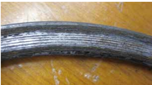
Figure2 Oxidation loss of expanded graphite from a spiral wound gasket
