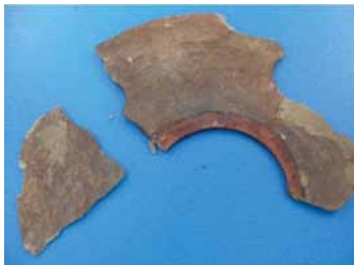
Figure5 压缩板的硬化开裂
