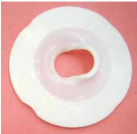
Figure6 Deformation of a fluoro-resin sheet gasket
