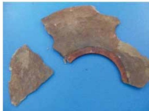
Figure5 Cracked joint sheet gasket due to hardening
