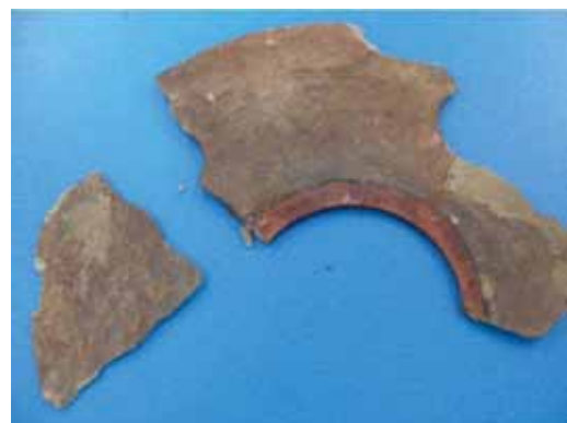
Figure5 Cracked joint sheet gasket due to hardening
