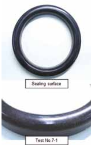
Figure9 Specimen after Test No. 7-1 leakage tests
