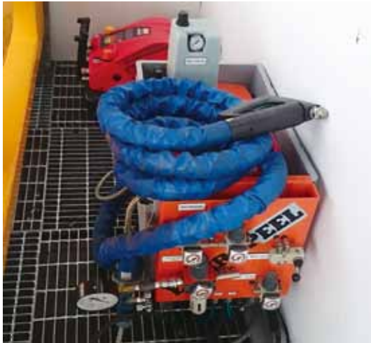
Figure4 Special rust-proofing operation unit
