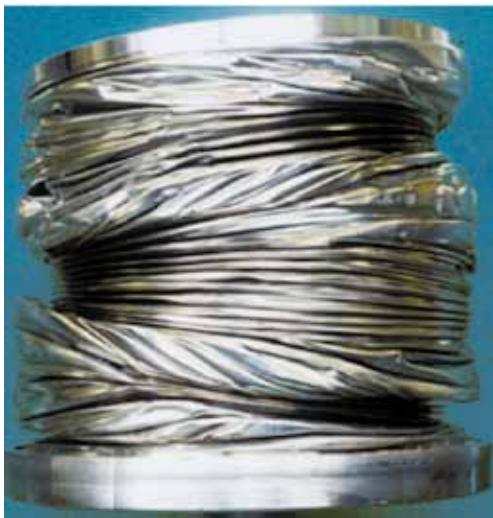
Figure6 Breakage due to buckling of Bellows
