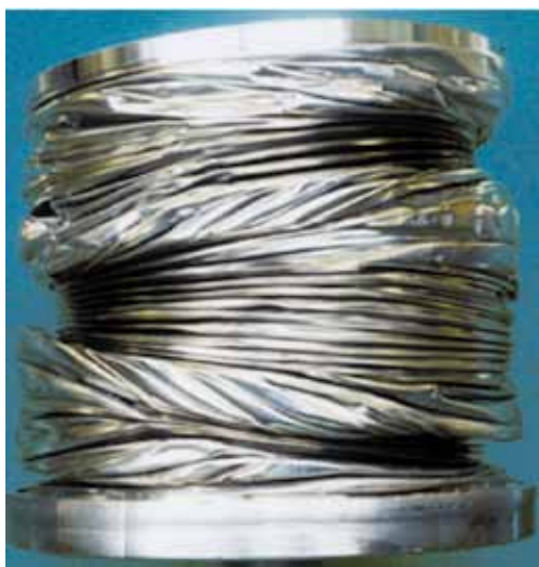
Figure6 Breakage due to buckling of Bellows
