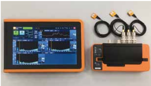
Figure1 External appearance of the vibration detection maintenance system Left : Tablet Upper right : Sensor (Approximately 2cm square) Bottom right : Wireless dock (amplifier)
