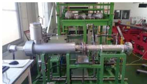
Figure1 Educational hands-on training equipment (The left side is the high temperature part, the right side is the low temperature part)
