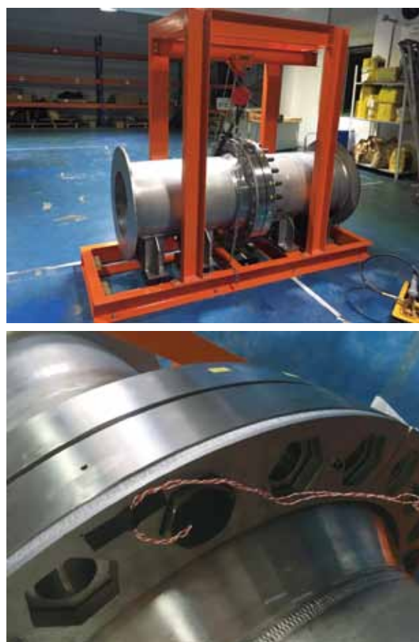
Figure1 Experimental equipment of 24-inch pipe flange connection
