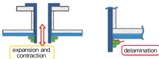
Figure14 Nozzle activity and loss examples due to temperature change
