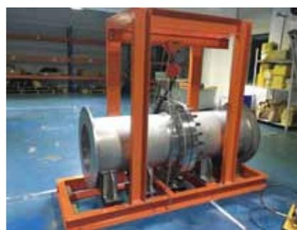
Figure2 試験治具(JPI Class300 24inch)
