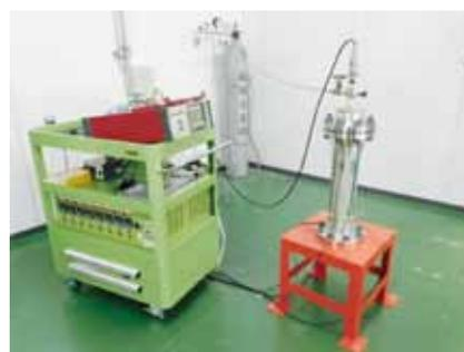
Figure1 試験治具(JPI Class150 4inch)
