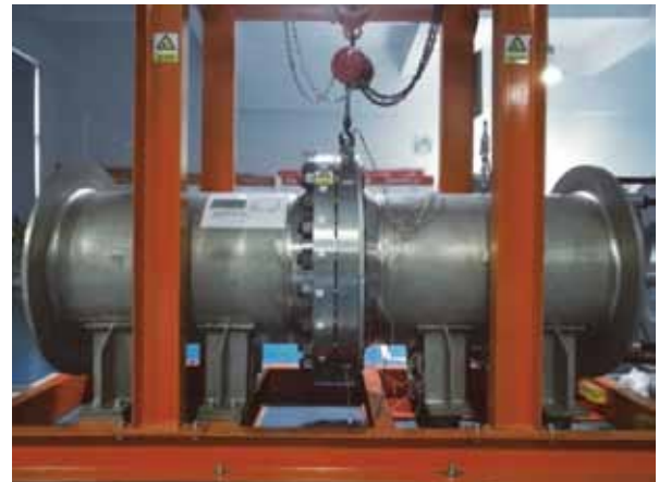
Figure1 Experimental setup of 24" pipe flange connection
