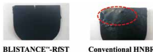
Figure7 Comparison of test specimen surfaces after refrigerant immersion test
