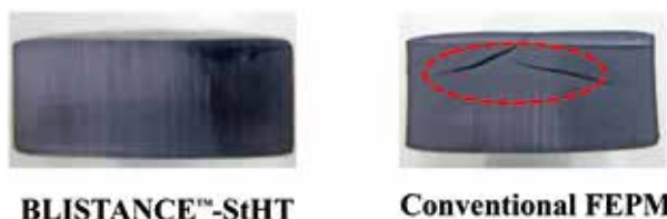
Figure6 Cross-section of test specimen after 72h of compression in 230°C steam
