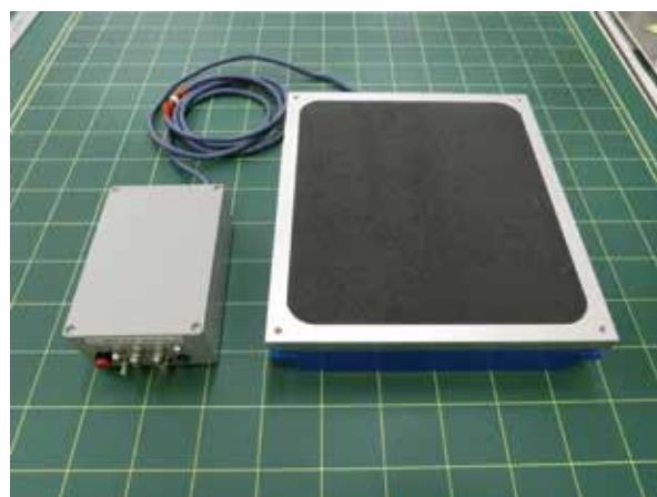
Figure6 Developed mat sensor system
