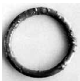
Figure2 Example of an O-ring where blisters have occurred
