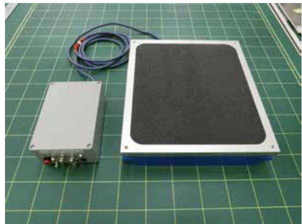
Figure6 Developed mat sensor system
