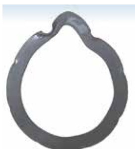
Figure4 Case of deformity due to uneven tightening (insufficient tightening in a section)
