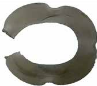
Figure2 Case of gasket blowout due to insufficient tightening
