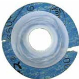
Figure3 Case of compression failure due to excessive tightening
