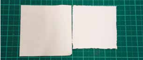
Figure2 Difference in thermal shrinking of PTFE nanofiber nonwoven fabric (left) and ePTFE (Right)
