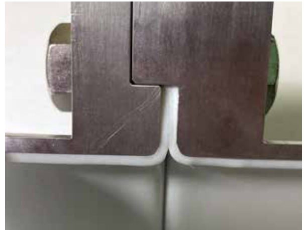
Figure4 Photograph of junction after tightening
