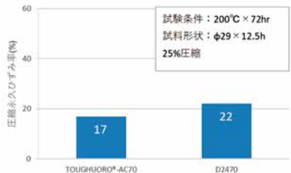
Figure5 TOUGHUORO ® -AC70の圧縮永久ひずみ率
